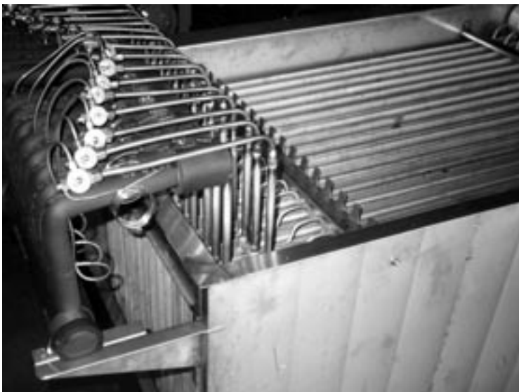
Fig. 61-2 Typical PLATECOIL banks used as falling film heat exchangers.
